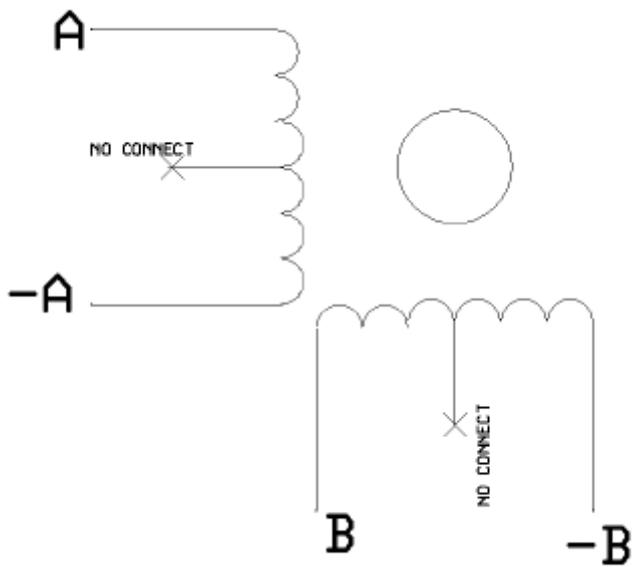
Eight-wiring step motor
