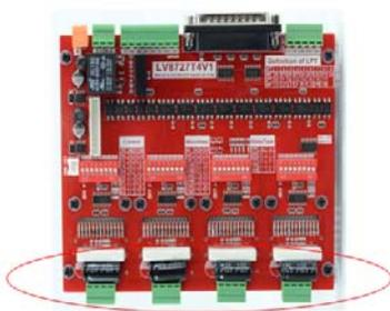
2. As picture, if you connect or break control interface of step motor during turning on power, the red button RESET in mach3 need to be flickering. (The red button of RESET has two states, flicker and stop flicker. You can switch two states by clicking the red button of RESET.) If not, the chip damage possibly.
