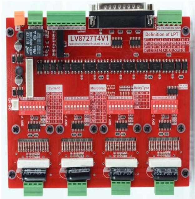
1. Can drive four 4A stepper motor at the same time and have the fifth axis extension interface.
