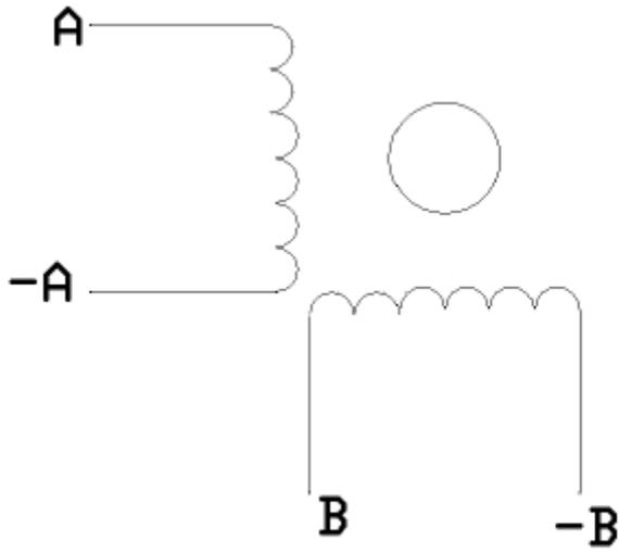
Six-wiring step motor
