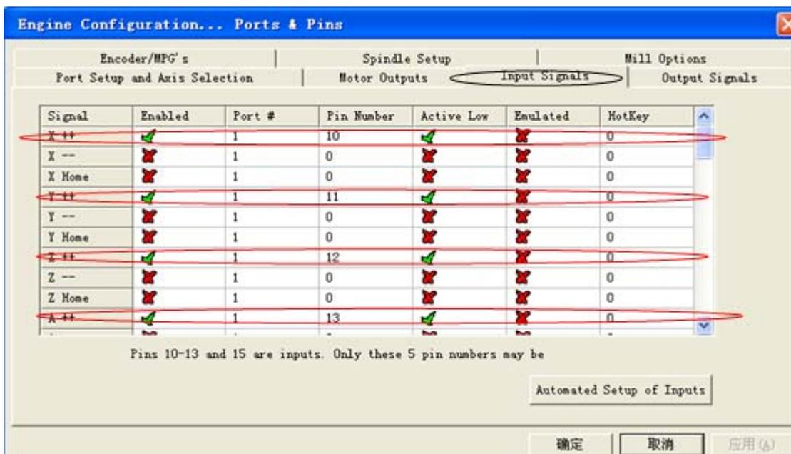
According to your need, you can select relevant functions, include up and down limit of XYZAB5 axis, Home zero point of XYZAB5 axis, PROBE tool setting, and ESTOP— urgent stop and others.
