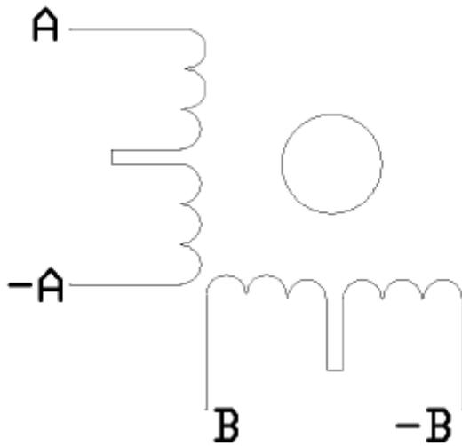
+A , -A , B and -B of step motor take turns to connect A+, A-, B+ and B- of the LV8727.
