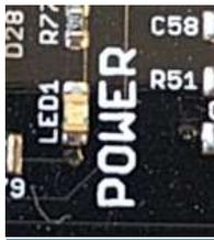
LED1: indicates that the external power is connected, this means that 24V and 5V are available.
